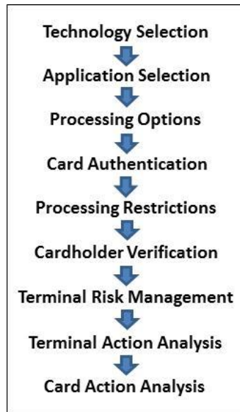
Figure 3. Processing Steps for an EMV Contact Transaction
